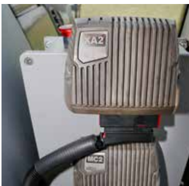
Centralina elettronica Parker programmabile per gestione completa dei comandi. Innovativo software "No stress control" con comando automatico combinato bracci primario, secondario e telescopico. Parker programmable control unit for full management of the commands. Innovative software "No stress control" with automatic combined control for primary, secondary and telescopic arms.
