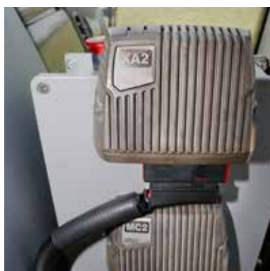
Centralina elettronica Parker o Danfoss programmabile per gestione completa dei comandi. Parker or danfoss programmable control unit for full management of the commands.
