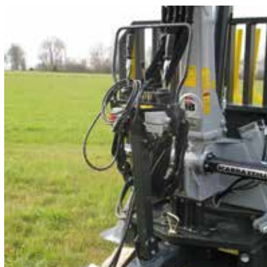
Posto guida a terra con distributore elettroidraulico. Driver's seat on the floor with electro-hydraulic distributor.
